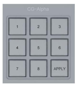
The hardware shortcut key on the control panel can be used to APPLY the effect to the PGM window more quickly. Click the corresponding serial number to generate a preview and then click Apply to apply to the PGM
