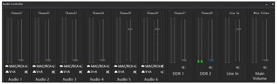
Click the horn button on the software to pop up the eight-channel audio controller. This function is mainly used for the adjustment of NDI and STREAM audio of each signal source channel. The MIC and stereo audio are subject to the equipment mixer
