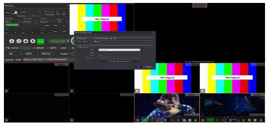
In push mode, a mobile phone or any device with the push function can be used to push the stream in the LAN. According to the push address in the push mode, the push stream can be sent to the device as a signal source to switch the broadcast. The following picture shows the mobile phone after pushing the stream.
