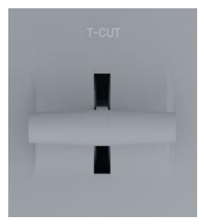
T-push rod: The T-push rod is a manual transfer mode, and the PGM and PVW switch is completed with WIPE or fade in and fade out effects
