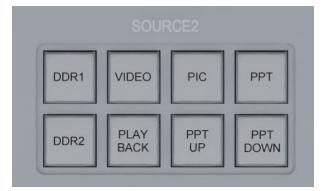
Fast switching of local materials; After connecting the software, you can use this function to control the playback of videos, pictures and PPT in the local materials in the software;
