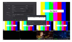
Search for the NDI signal source in the LAN and configure the corresponding channel address. The current channel is channel 1, so select Channel 1. The NDI signal can be generated as shown below
