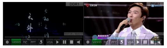
The DDR window of the software is mainly used to add local pictures, videos, and PPT as signal sources to switch the broadcast. Recommended formats of live broadcast images are JPG and BMP. Resolution: 1080P
