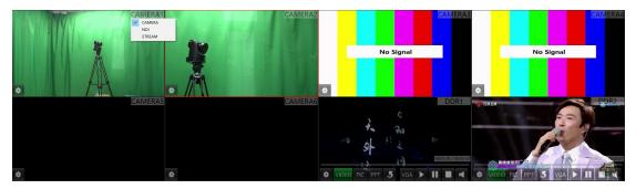
The above picture shows the eight-channel signal premonitoring interface. Since the device with the software installed cannot access the camera, the signal can only use NDI and STREAM modes, and DDR1 and DDR2 are independent footage Windows.
