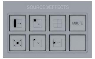
WIPE Transition effects selection key set: 6 fixed WIPE effects selection keys, the user directly on the panel to select the WIPE effects according to the icon.
