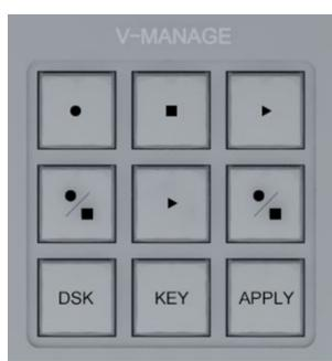
The first row is the software recording, stop, and live function shortcut keys, and the second row is the local recording and stop, live, and NDI recording
