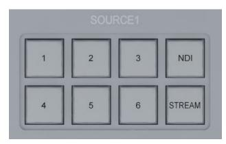
After connecting the software, you can quickly switch the premonitor window mode. Select the window value and press the NDI or STREAM key to quickly switch between NDI and STREAM
