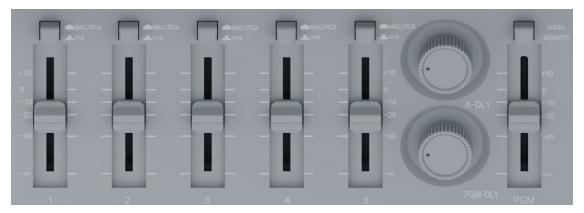
1 to 5 channel audio gain adjustment, corresponding to the backplane 1-5 audio input, MAC/V+A digital/analog audio switch key, audio delay, PGM audio gain adjustment. PGM Mute with one click $_{\circ}$
