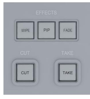
WIPE: Switch on transfer effects mode and use with WIPE transfer keys
