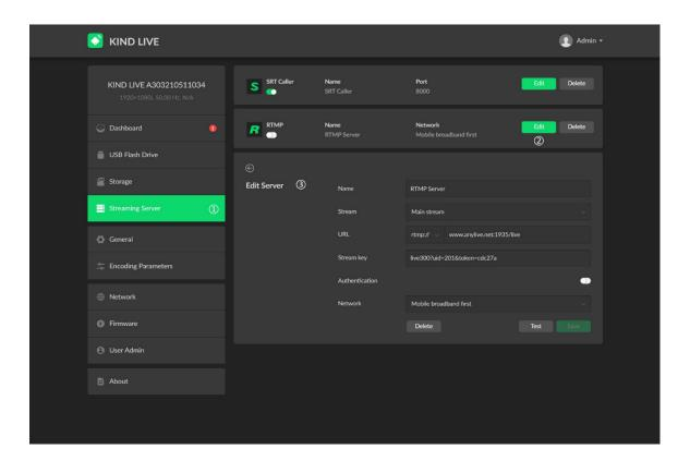
Fill in the relevant address in the SRT control panel according to the steps below. Click Test to check whether the connection status is normal
