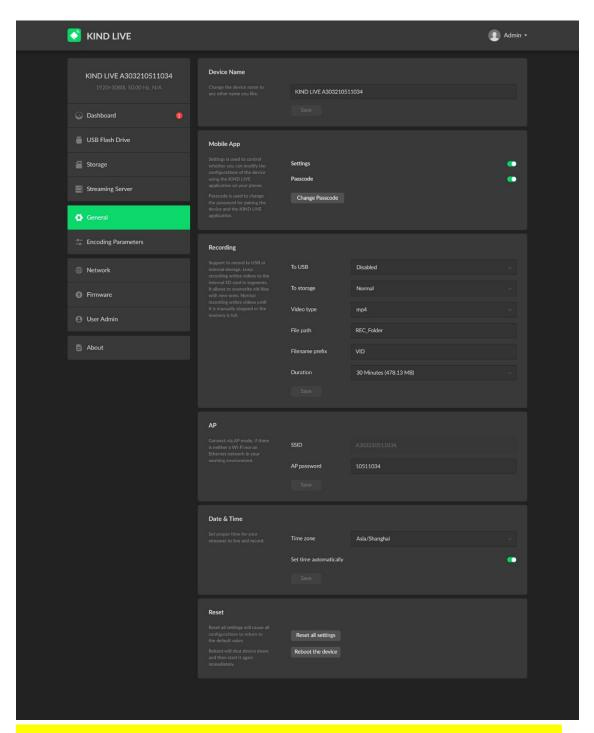
Note:TF storage and USB storage can only choose one, the setting can not be opened at the same time, otherwise it will cause read and write errors
