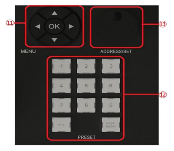
① Camera menu function: First click the OK key to display the menu of the POC camera, and the built-in functions of the camera can be adjusted through the up and down left and right buttons.
